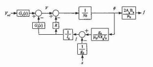
Fig. 5. Schematic view of the actuator/amplifier/rotor interaction. Eddy currents are not indicated
