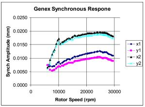
FIGURE 9. Measured synchronous displacement amplitude from full speed run of machine.
