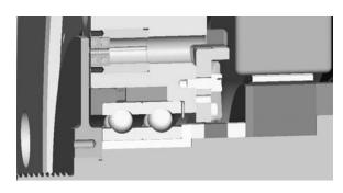
FIGURE 2. Cross-section showing radial/thrust backup bearing.
