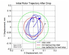
FIGURE 10. Measured rotor/housing displacement orbit after rotor drop at 23,000 rpm.
