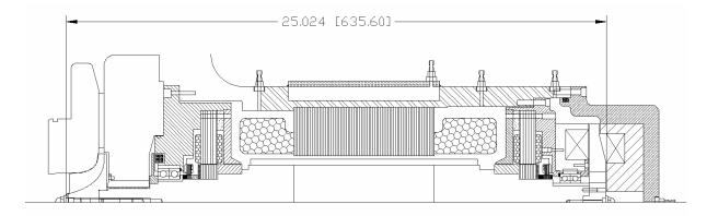
FIGURE 1. Cross-section of expander generator with nominal 114 mm (4.5 in) wheel.
