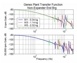
FIGURE 3. Comparison of predicted plant transfer functions for three different expander wheels.
